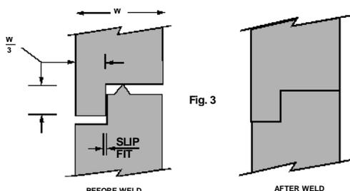
**Figure 4.** A tongue and groove joint usually has the capability of providing greatest strength. The need to maintain clearance on both sides of the tongue, however, makes this more difficult to mold. Draft angles can be modified concurrently with good molding practices, but interference between elements must be avoided.
