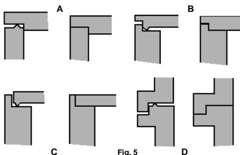
**Note:** When the interference joint is used, weld strength of crystalline materials approaches 95% of parent material strength, as opposed to 40-70% when energy director is used. The interference joint permits interaction between the two surfaces during the entire melt cycle by exposing more and more surface area as the two surface planes interfere under ultrasonic and clamp force.
