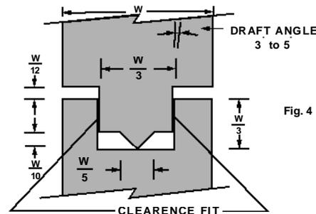
**Figure 5.** Illustrates basic joint variations suitable for ultrasonic welding. These are suggested guidelines for typical joint proportions. Specific applications may require slight modification. Practical considerations suggest a minimum height of .005" for the energy director. Where height greater than .020" is indicated, two or more directors should be provided with the sum of heights equalling the formula dimensions.
