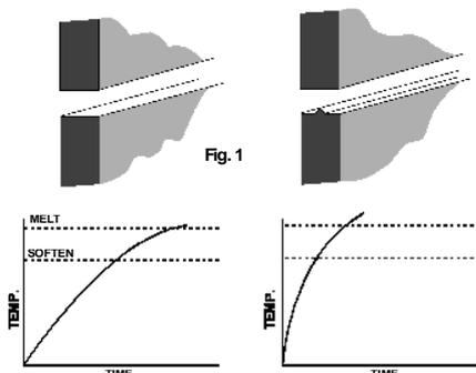
**Figure 2.** Shows a simple butt joint modified with energy directors showing desired proportions before weld and indicating the resultant flow of material. Parts should be dimensioned to allow for the dissipation of the material from the energy director throughout the joint area as illustrated.
